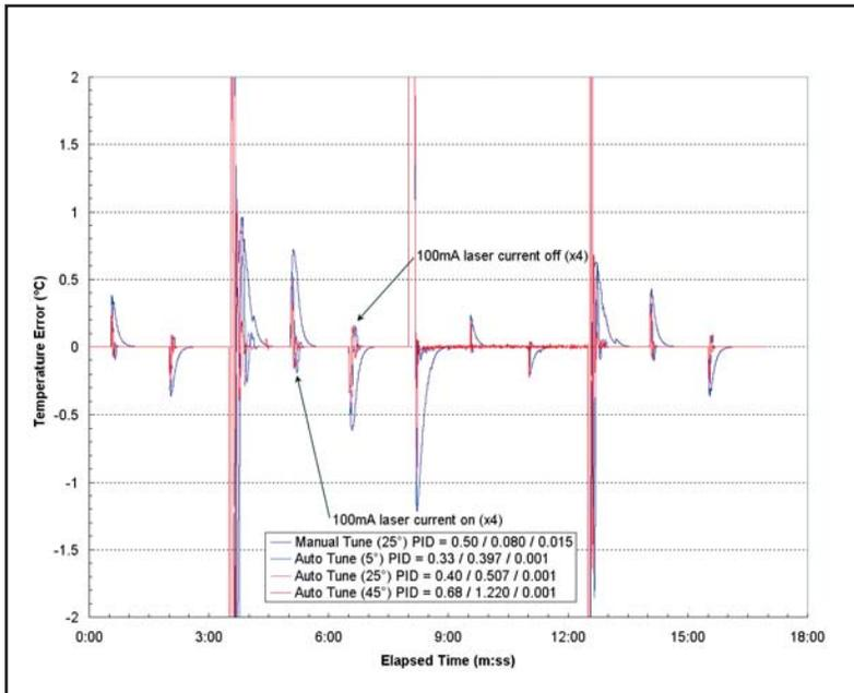
Figure 8. Temperature Error
