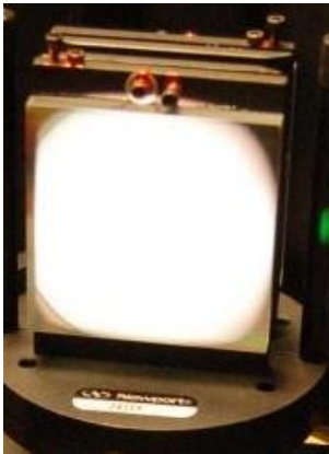
Figure 22: Grating Correctly “Filled” with Light
