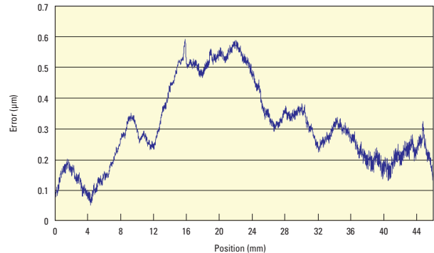
Accuracy of a XMS50-S stage after linear error correction. The data was taken dynamically at a rate of 10 kHz while the stage was moving at a speed of 100 mm/s. Both the encoder and the interferometer positions were acquired by an XPS motion controller with a latency of less than 50 ns between the different signals.
