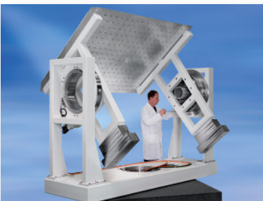
◀ 2-Axis gimbal with custom RTM660 stages for load capacity up to 2000 N used in remote sensing instrument test and measurement.
