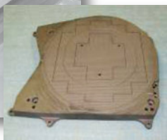
◀ Support for 200 & 300 mm wafers, <2% backside contact, 100 nm flatness per 50 mm 2 area.
