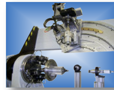
▲ Multi-axis SOC using autocollimator.
