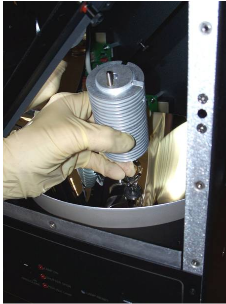
Photo 20: Heat sink unscrewed from socket
