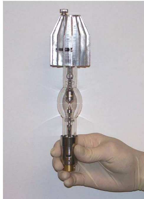
Photo 10: 1kW lamp with heat sink attached
