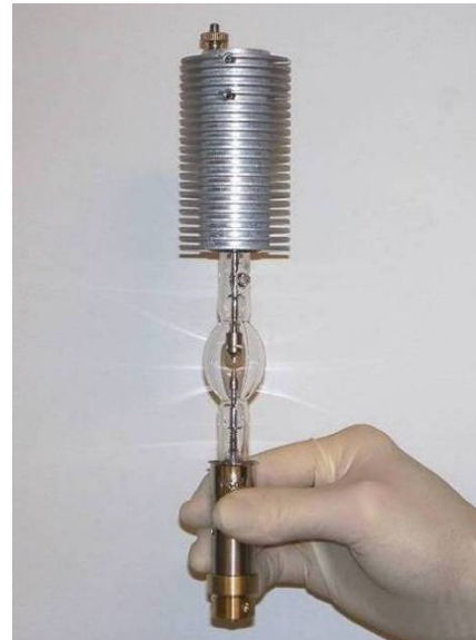
Photo 9: 450W Lamp with heat sink attached
