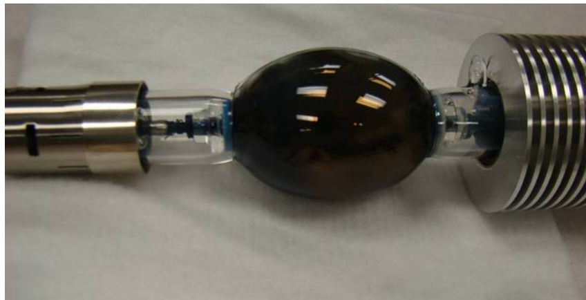
Photo 23: Lamp run under reverse polarity
