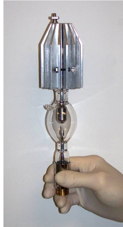
Photo 11: 1.6 kW lamp with heat sink attached
